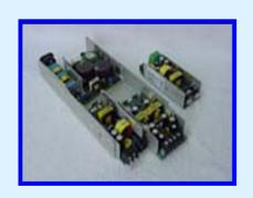
Custom power supplies in single and multiple outputs from 50W to 750W
